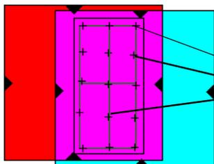
Put orientation tie points on common features in the corners, edges and center lines of the stereo overlap area.
