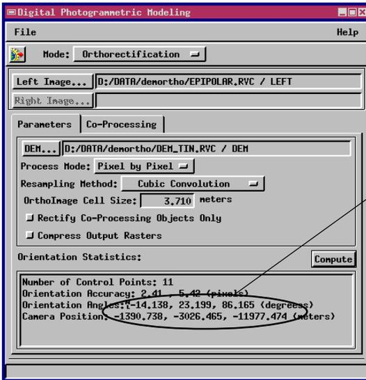
In this example, the first two computed camera rotation angles deviate radically from the ideal 0, 0 (“straight down”) orientation, so the process cannot proceed. As a side effect, the Camera Position values show a position *below* the surface. Even small errors and inaccuracies in georeference and orientation control can cause these values to jump out of useful ranges.
