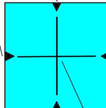
The **Principal Point** is the address of the cell where lines that connect opposite fiducial marks intersect.
