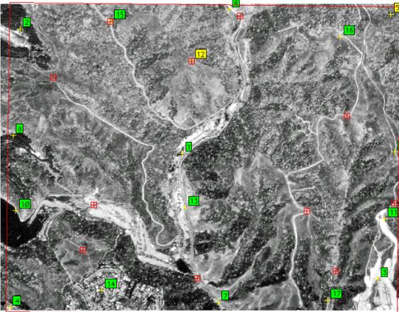
The red overlap area box should not be skewed and should have right-angle corners.
