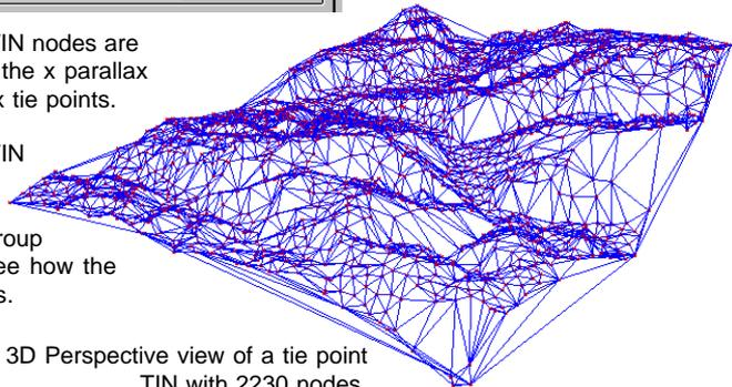
3D Perspective view of a tie point TIN with 2230 nodes.
