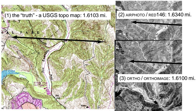
Not every test measurement compared as well. Nevertheless, all the ORTHOIMAGE measurements were closer to the values from the topo map than the RED146 values were.
