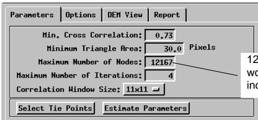
12,000 nodes is enough for orthophoto work. To get sharper surface detail, increase the maximum to 40,000 or more.
