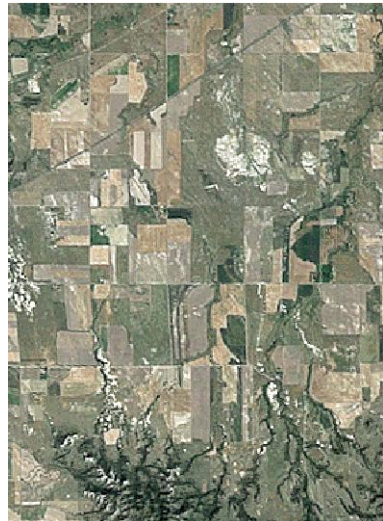
Same area with 3 x 3 Volterra filter applied (displayed with auto-linear contrast), showing enhanced detail.
