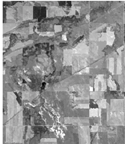
Same area with 3 x 3 CS filter applied (displayed with auto-linear contrast). Field boundaries and linear features are clearer.
