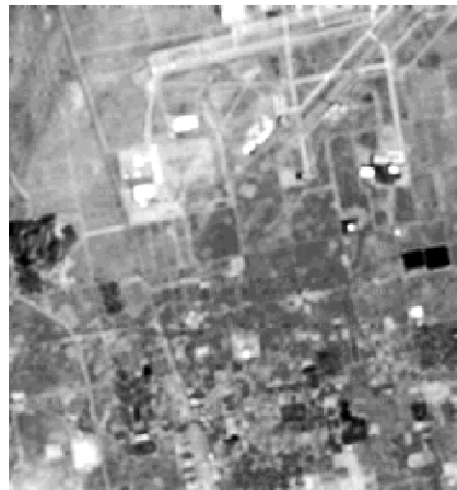
Same part of image with 3 x 3 low pass filter applied (auto-normalized contrast). Striping is reduced, but small features are slightly blurred.
