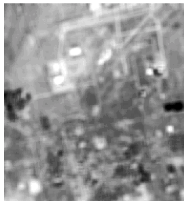
Upper right part of raster object TM3NOISY with 7 x 7 Low Pass filter applied (auto-normalized contrast). Spatial averaging has greatly reduced image detail.
