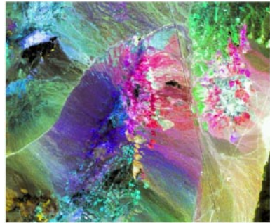
RGBI display of the first 4 MNF components (3 = Red, 2 = Green, 4 = Blue, 1 = Intensity).
